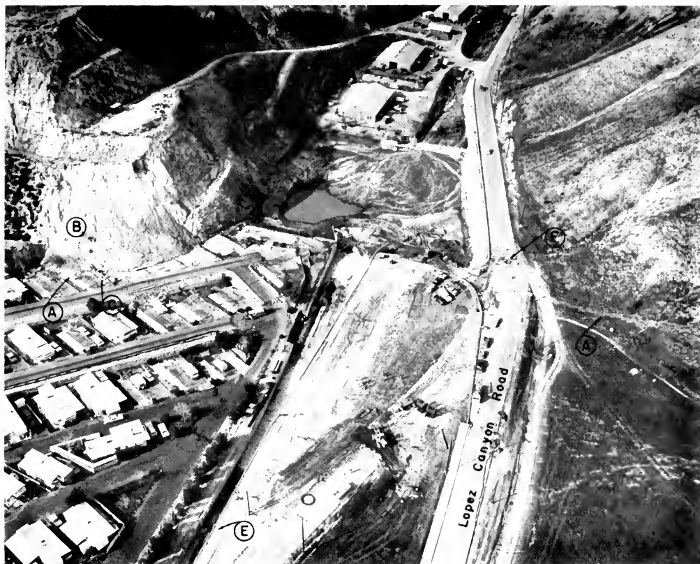
Photo 2. Low-altitude oblique aerial photo of the mouth of Lopez Canyon. Lettered localities: (A) scarp of the Tujunga fault segment; (B) rockfall caused by earthquake; (C) site of trench 8 in Blue Star Trailer Park; (D) bedding in Madela Formation; (E) damage to flood control channel; (F) 38 cm (15-inch) left-lateral displacement of white line on Lopez Canyon Road. Photo courtesy of the Los Angeles Department of Building and Safety.
